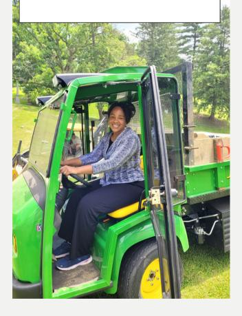
After waiting almost a year, we received our John Deere Pro Gator! (see pic above) It is a mini dump truck. This heavy duty equipment keeps our small grounds crew efficient, has four wheel drive, fits perfectly in between the narrow lot rows, has wide turf tires that reduce damage to the ground, and it hauls up to 4000 pounds! We are thrilled to have this piece of equipment.
